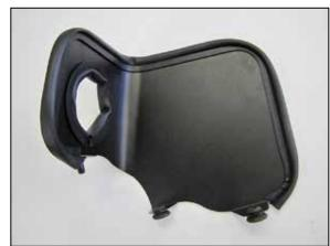
8. Install the 13.5" edge trim into the hole of the heat shield and install the 36" edge trim around the outside of the heat shield as shown.
