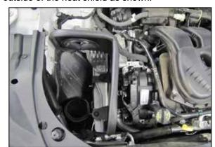
9. Install the heat shield into the vehicle so the mounting grommets and studs engage.
