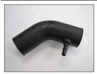
10. Install the vent fitting into the K&N® intake tube as shown.
