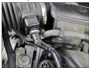
3. Release the locking tab and disconnect the crank case vent line from the factory intake tube.
