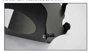
6. Install the air box mounting stud onto the K&N $^{\!\otimes}$  heat shield using the provided hardware.
